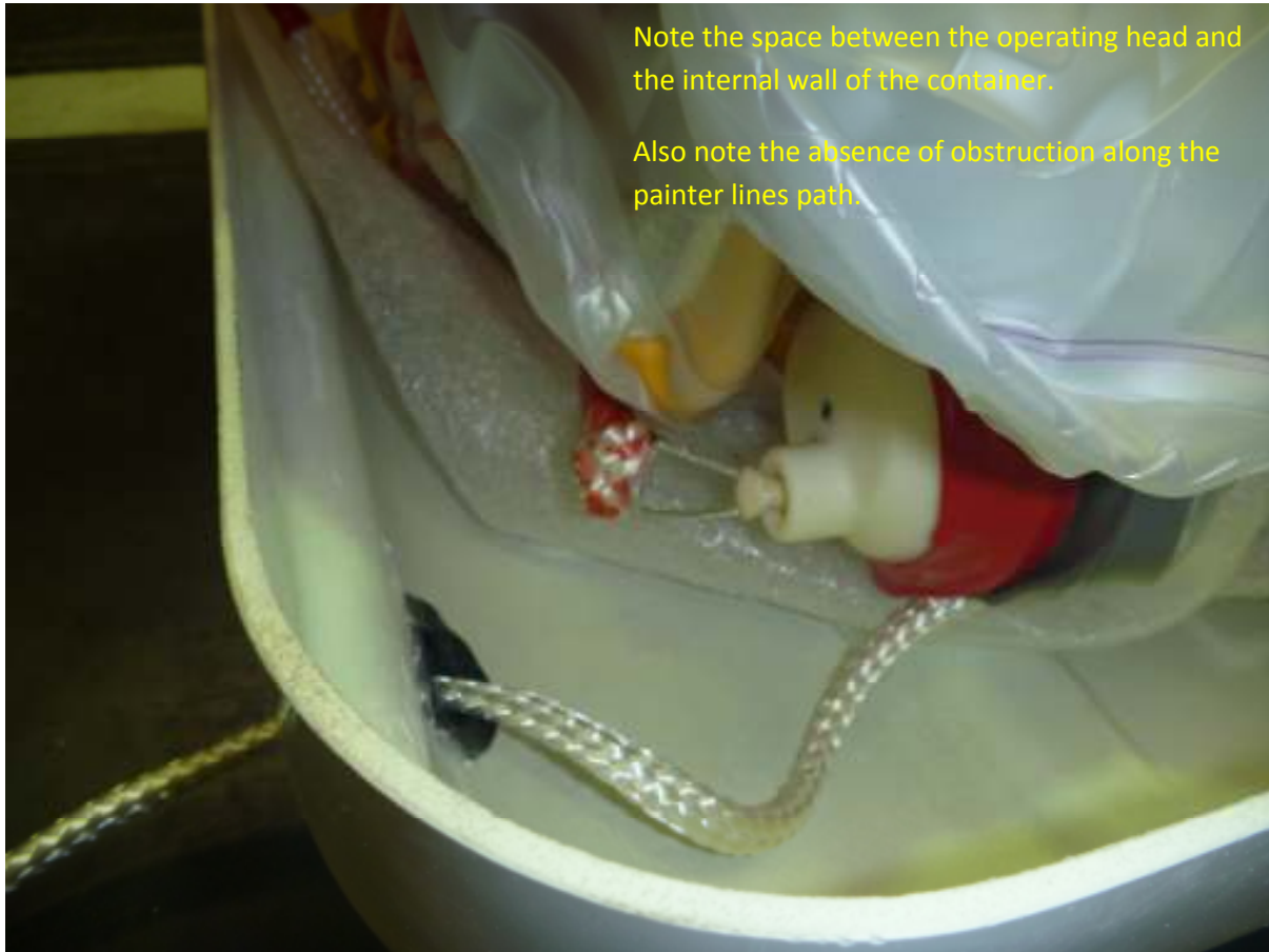
Fig 3 – Vacuum Packed Liferaft Located Inside Container
